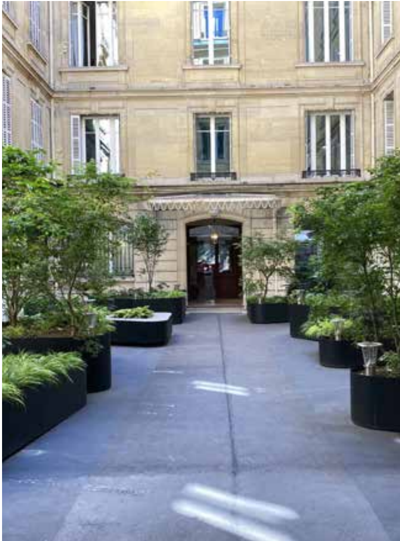
Paris 8 th 5 mm aluminium welded planter, watertight base, RAL 9005 textured finish. Moabi seat.
